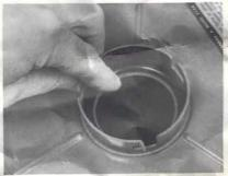
The new "O" ring found in the wick package should be inserted in the fount top.
