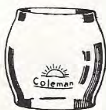
690-058 (660) PYREX GLASS GLOBE Bulge type. Use on Lantern 237A. 5 3/4 inches diameter by 5 1/4 inches high.
