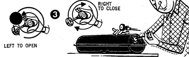
(3) two complete turns to the left. Place thumb over the small hole in handle and pump 35 to 50 full strokes of air into the tank. Then turn pump plunger handle to the right and tighten firmly.
