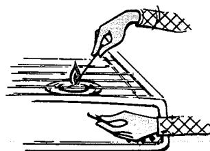
**THE STOVE GENERATOR** changes liquid fuel to a vapor. Eventually it may fill with carbon so no fuel can be forced through it. Avoid problems by keeping a spare generator, No. 412-262 on hand.
