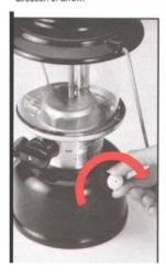
■ Remove FUEL CAP. Use a funnel or suitable filling device and fill with clean, fresh fuel. Lantern must be in a level position.
